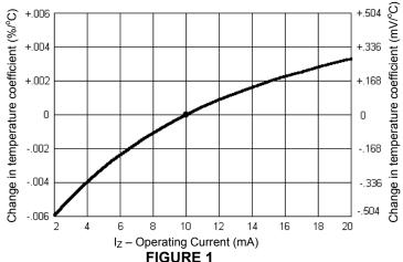
TYPICAL CHANGE OF TEMPERATURE COEFFICIENT WITH CHANGE IN OPERATING CURRENT.
